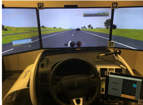
11 12 Figure 1 Driving simulator and NDRT
